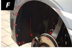
Screws holding the wheelhouse cover.
