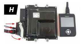
VCL connected for decoding.
